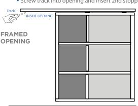
Note: GLIDE and track must be installed as one unit. Additional help may be required. Any adjustments in height must be completed outside the track.
